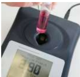
Inserting the phosphate sample into the photometer
